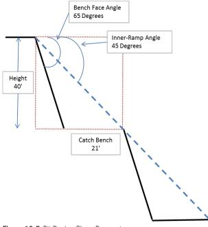
Figure 16-5. Pit Design Slope Parameters
