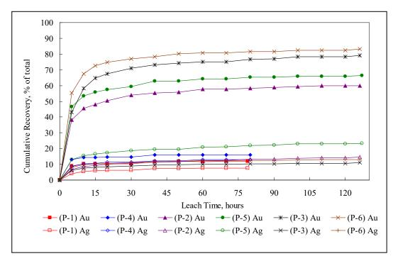
Figure 13-1. Gold and Silver Leach Rate Profiles, Column Percolation Leach Tests (From Medina, 2012)
