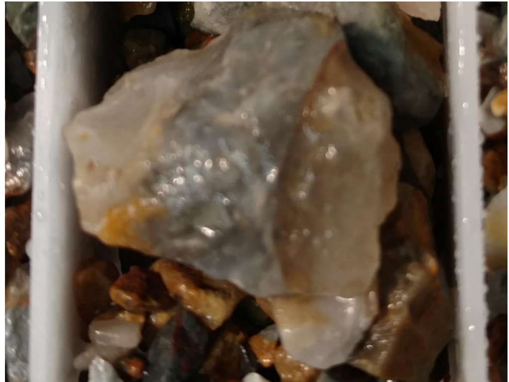
Quartz-cemented hydrothermal breccia with minor gray sulfide & oxidized pyrite within wider quartz vein
